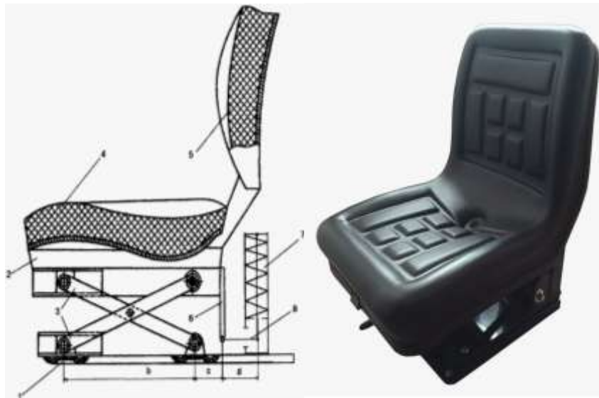
1 – base; 2 – frame; 3 – guide device (type "scissors"); 4 – cushion; 5 – back; 6 - bracket; 7 – shock absorbing device; 8 – base plate
